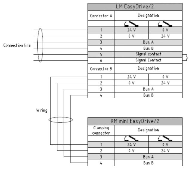
Deviating for BUS-capable drives! See separate BUS manual!
