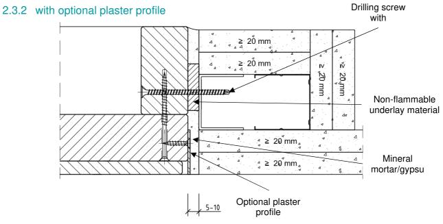
Fill the frame and mounting frame over the entire surface and all around!
