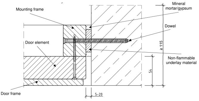
Fill the mounting frame over the entire surface and all around!
