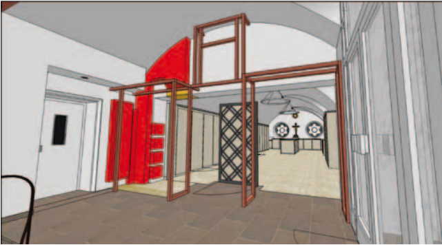
Steel scaffolding to form the drywall construction
